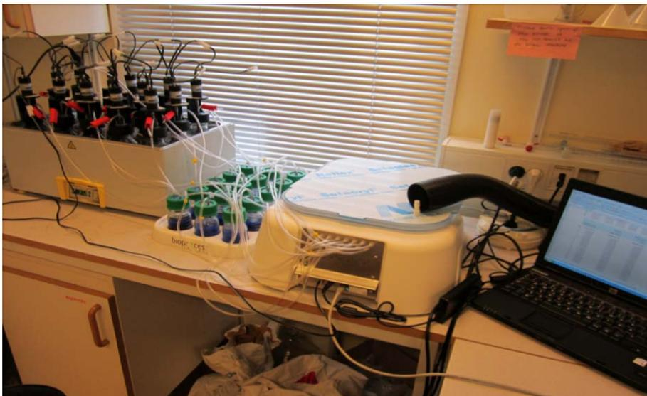
**Figure 3.** Picture of the *Automatic Methane Potential Test System* (AMTPS II) at Hammarby Sjöstadswerk (Almkvist, 2012).
