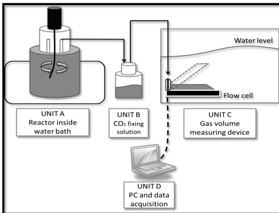
**Figure 4.** Schematic view of the experimental setup (Rodriguez, 2011)
